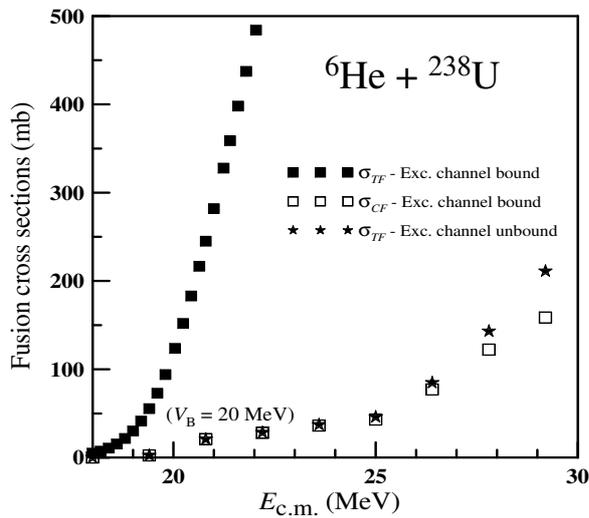
FIG. 1: Total fusion cross section of ref. [18] (solid squares) compared with that of the present work (stars). The present calculation uses the same potential, channel coupling and simplifying assumptions of [18]. The basic difference is that here the contribution from incomplete fusion uses the tunneling of the  ${}^4\text{He}$  fragment, rather than the full  ${}^6\text{He}$  projectile. For comparison, the complete fusion cross section of [18] is also shown (open squares).
