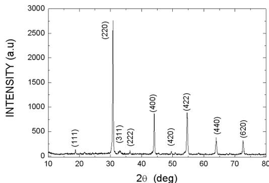
FIG. 1: Diffraction pattern of SYSO polycrystalline target.
