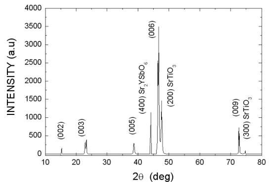
FIG. 2: Diffraction pattern of YBCO/SYSO/STO films.
