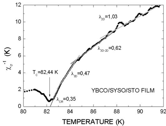
FIG. 4: Fluctuation regimes in plot of the inverse of logarithmic temperature derivative for YBCO/SYSO/STO thin films.
