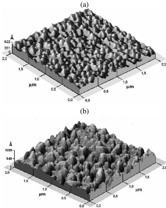
FIG. 3: AFM photograph of (a) SYSO/STO and (b) YBCO/SYSO/STO.
