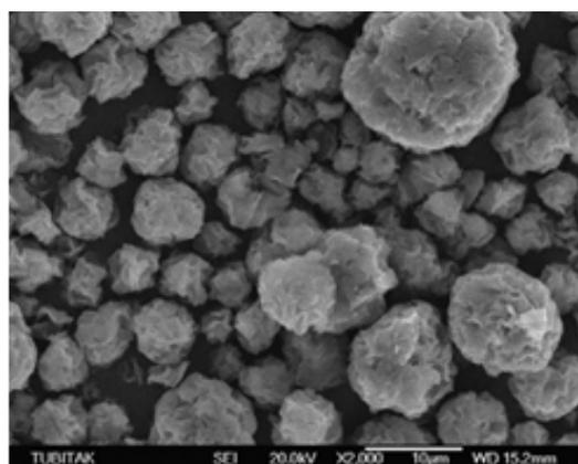
**Figure 6.** SEM of natural montmorillonite (MMT-Na), at a magnification of 2000x. Source: Sarier et al.<sup>[22]</sup>.
