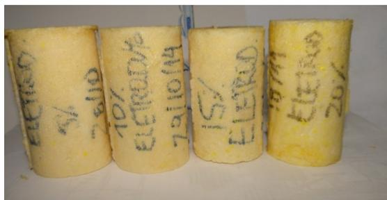
**Figure 2.** PU/PVC composites with 5%, 10%, 15%, and 20% conduit.
