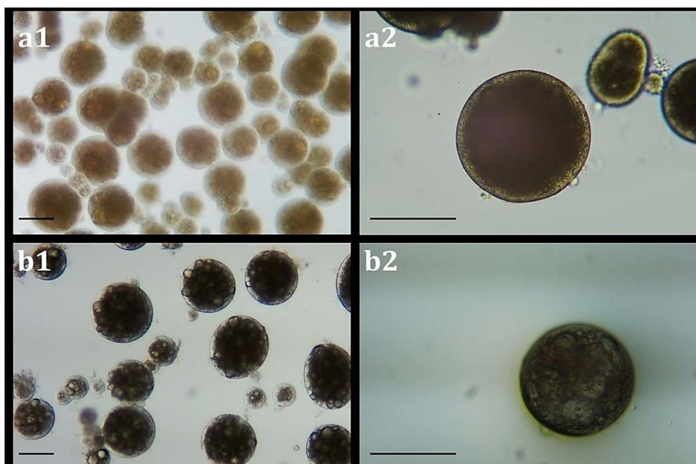
**Figure 2.** Optical microscopy images of synthesized microcapsules: (a1) gelatin/gum arabic microcapsules containing fatty acids from microalgae 40X and (a2) 100X; (b1) gelatin/gum arabic microcapsules containing *A. vera* oil 40X and (b2) 100X. Scale bars = 100 µm.
