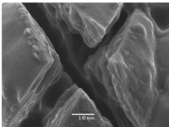
**Figure 3.** SEM image of a ruptured microcapsule containing *A. vera* oil showing the wall thickness. Scale bar: 10  $\mu\text{m}$ .
