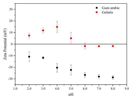
**Figure 1.** Zeta potential (mV) of the initial biopolymer's dispersions, gelatin and gum arabic, both at 2.5 wt%.
