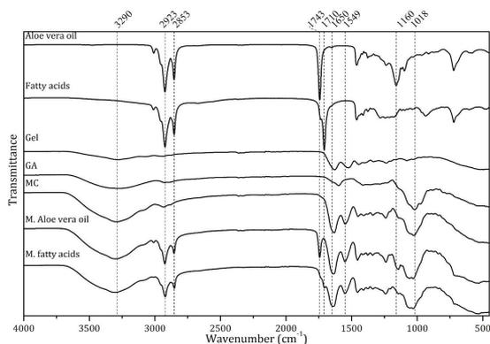
**Figure 5.** FTIR spectra of the core materials (Aloe vera oil and fatty acids), the shell polymers (Gel and GA), empty microcapsules (MC), and filled microcapsules with the respective material (M. Aloe vera oil and M. fatty acids).
