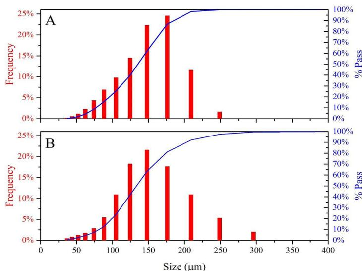
**Figure 4.** Particle size distribution obtained by laser granulometry: (a) microcapsules containing fatty acids from microalgae and (b) microcapsules containing *A. vera* oil.
