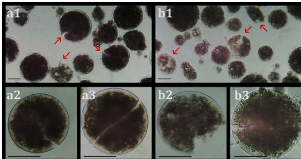
**Figure 6.** Optical microscopy images of gelatin/gum arabic microcapsules containing fatty acids from microalgae ((a1) 40X and (a2–a3) 100X) and microcapsules containing *A. vera* oil ((b1) 40X and (b2–b3) 100X) in 60% glucose solution for 1 h. Scale bars =100  $\mu\text{m}$ .
