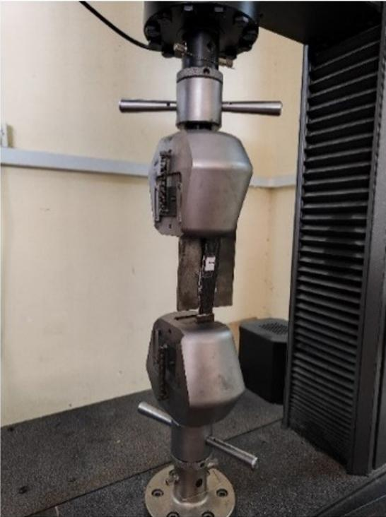
Figure 4. Peel test.
