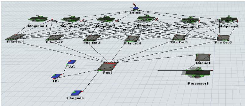
**Figure 2.** Overall view of the FlexSim model displaying the objects used. Source: elaborated by the authors.
