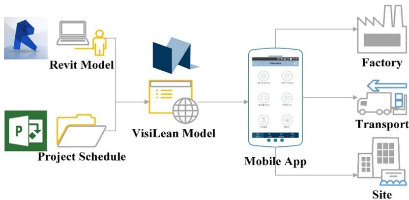
**Figure 2.** Prefabricated panel monitoring scheme.
