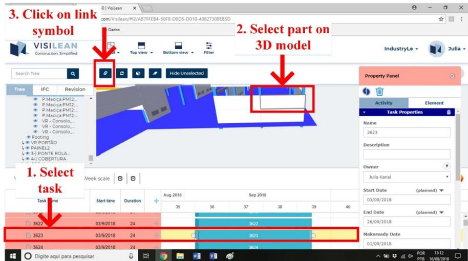
Figure 3. Link formation between the 3D model and schedule.
