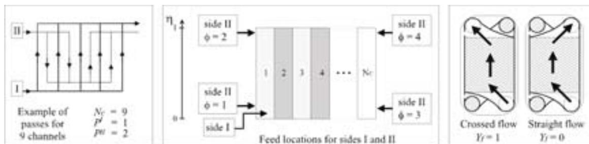
Figure 1: Spatial definition of parameters  $P^I$ ,  $P^{II}$ ,  $\phi$  and  $Y_f$ .
