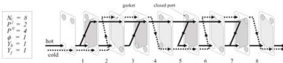
**Figure 2:** Example of configuration for a PHE with nine plates (eight channels).
