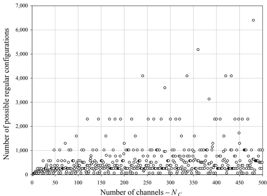
**Figure 3:** Number of possible regular configurations as a function of the number of channels.
