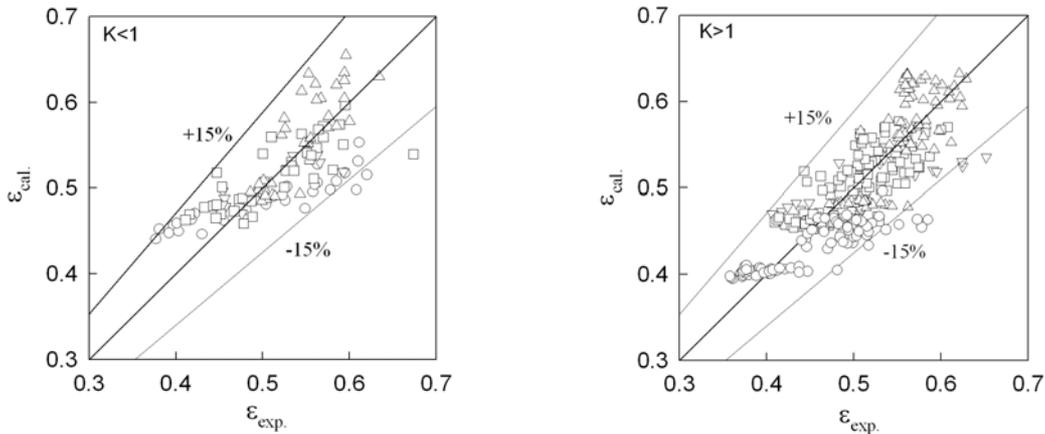
**Figure 7:** Comparison of prediction of  $\bar{\varepsilon}$  by Eq.(3) with the experimental values (○ millet; ▽ resin; □ sand; Δ glass beads)
