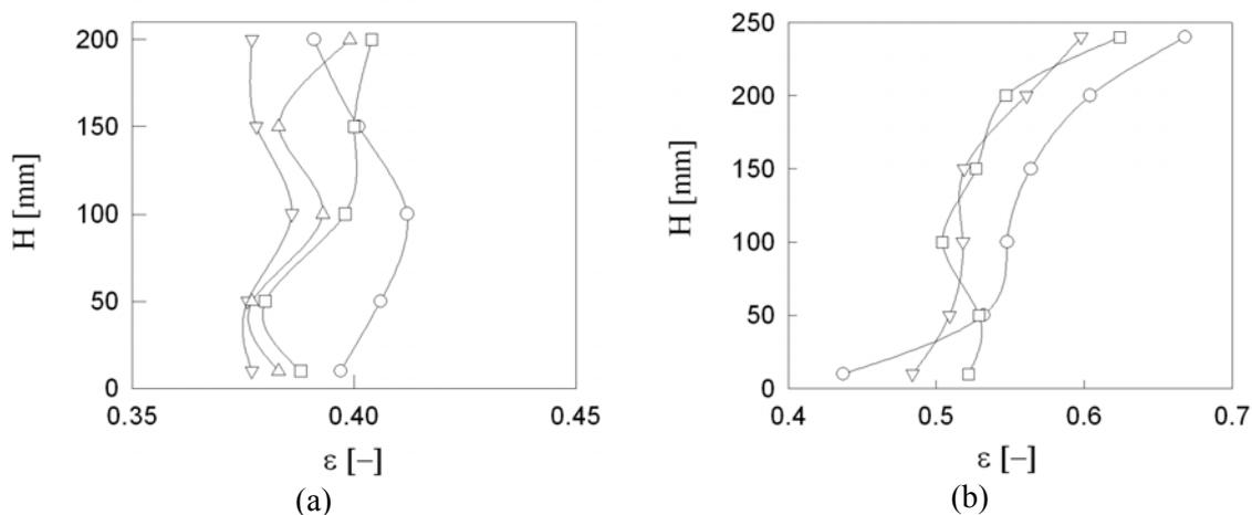
**Figure 2:** Axial distribution of bed voidage in a vibrating fluidized bed (a)  $u/u_{mf} = 1.10$ ; (b)  $u/u_{mf} = 1.80$ ;  $\circ$   $K=0$ ;  $\nabla$   $K=1.21$ ;  $\square$   $K=2.72$ ;  $\triangle$   $K=3.70$
