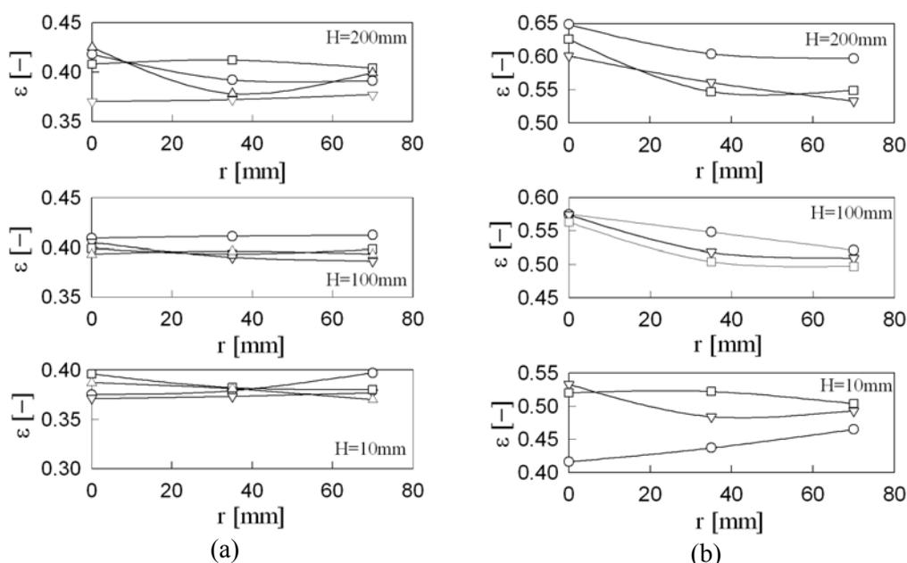
**Figure 3:** Radial distribution of bed voidage with vibration
