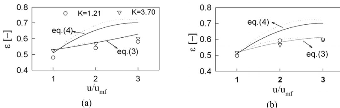
**Figure 8:** Comparison between prediction of overall bed voidage by eq. (3) and eq. (4) (Chevilank et al., 1979), (a) sand; (b) glass beads; Solid line:  $K=1.21$ ; dashed line:  $K=3.70$
