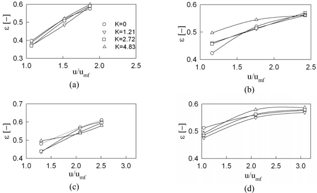
**Figure 6:** Relationship between bed average voidage and fluidization velocity (a) millet; (b) sand; (c) resin; (d) glass beads
