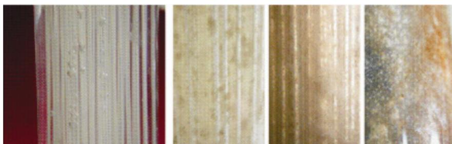
**Figure 6:** Biofilm accumulation on the surface of the MABR fibers - from left to right, 0, 7, 15 and 60 days of operation.
