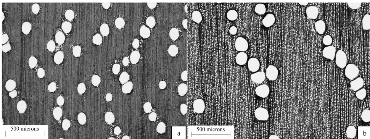
**Figure 2** – Photomicrographs of *Eucalyptus grandis* wood at age 21 years. a) Transverse section, fertilized wood b) Transverse section, unfertilized wood. Bar scale = 500 $\mu$ m.
