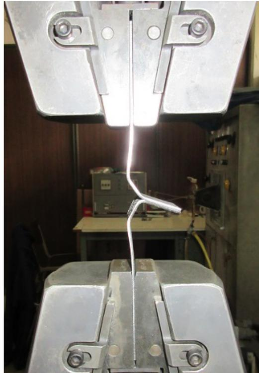
Figure 3. Placement of the specimens to perform the Peel test.
