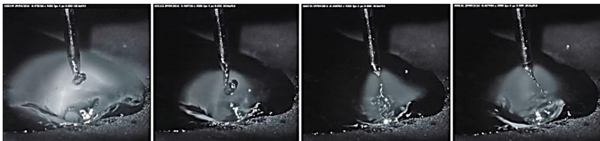
Figure 5. Rapid Arc metal transfer multiple-drop formation during the pulse period (high-speed films available on the LABSOLDA channel [26]).
