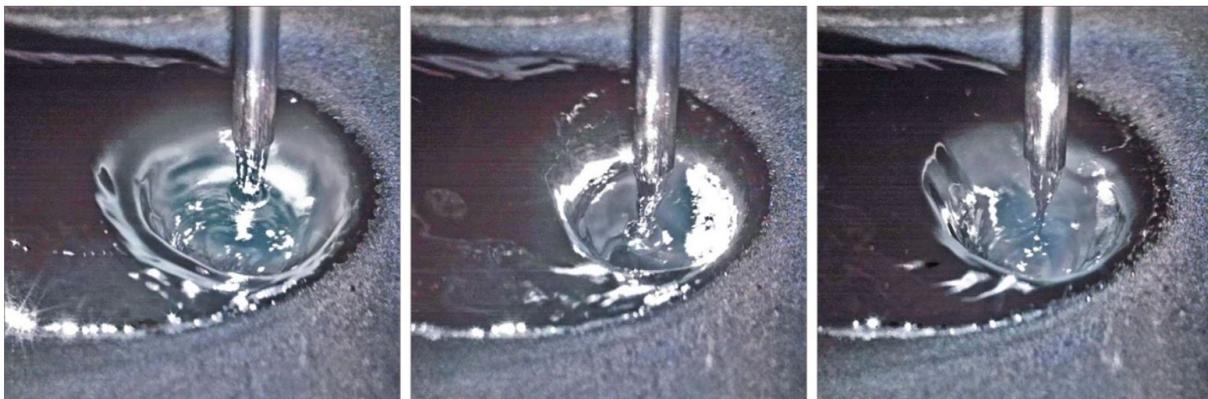
**Figure 2.** Crater created by arc pressure on the weld pool for tests carried out under bead-on-plate conditions.
