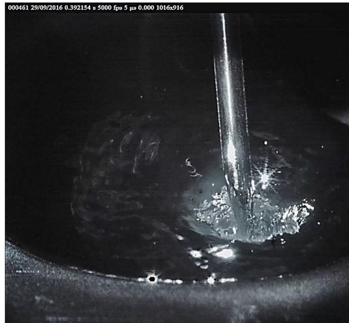
**Figure 3.** Crater instability during short circuiting, due to an inadequate inductance adjustment (high-speed film available on the LABSOLDA channel [24]).
