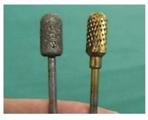
FIGURE 1: Carbide bur on right side and diamond fraise on left side
