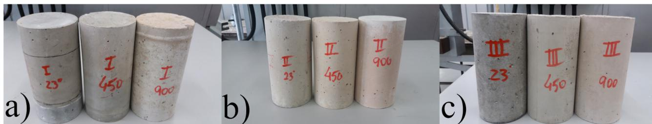
Figure 1: Images showing the color of the samples with composition 1 (a), 2 (b), and 3 (c), before (23 °C), and after heating at 450 and 900 °C. [Figura 1: Imagens mostrando a cor das amostras com composição 1 (a), 2 (b) e 3 (c), antes (23 °C) e após aquecimento a 450 e 900 °C.]
