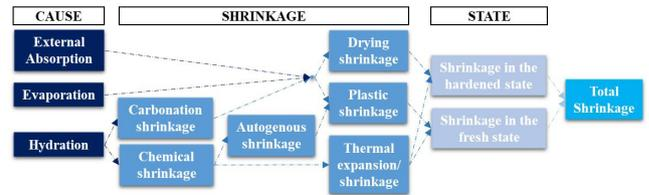
Figure 5: Scheme of interconnection between cause, type, and state for the shrinkage to which cementitious systems are subjected (adapted from [23]).
