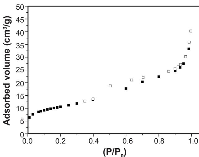
Figure 2: N<sub>2</sub> adsorption (filled square) and desorption (open square) isotherm of RAW-VER.
