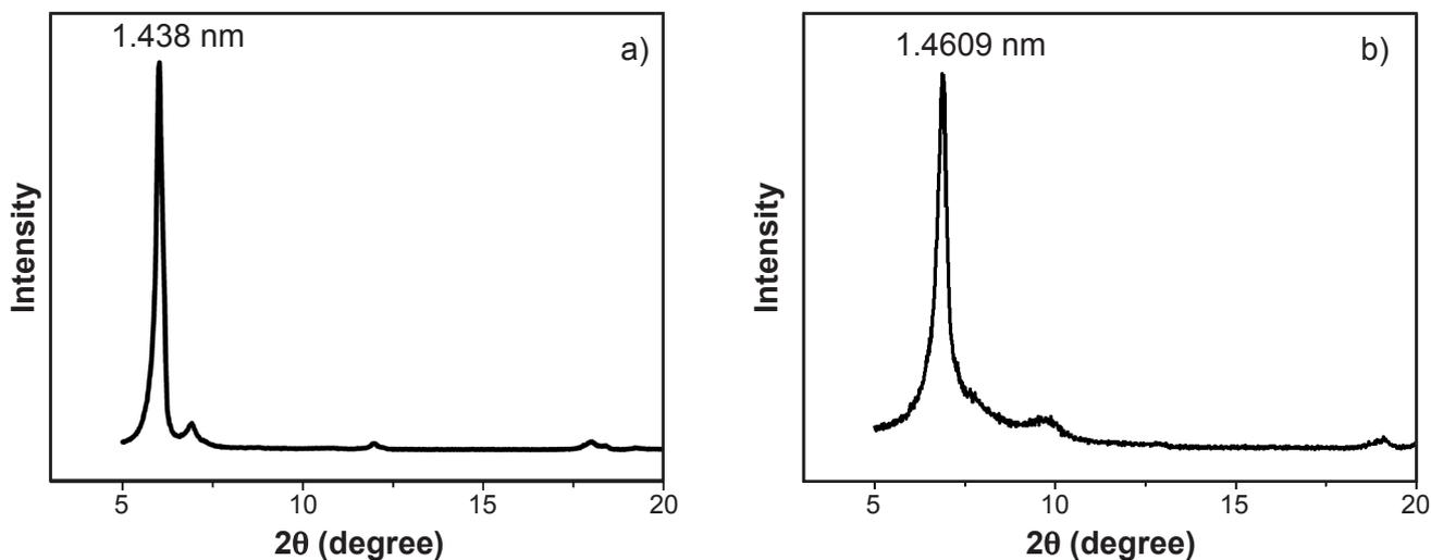
Figure 4: XRD patterns of vermiculite samples: a) RAW-VER; and b) VER-MW.
