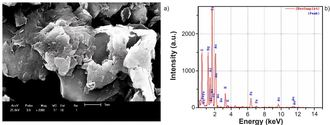
Figure 5: SEM image (a) and EDS spectrum (b) of RAW-VER.
