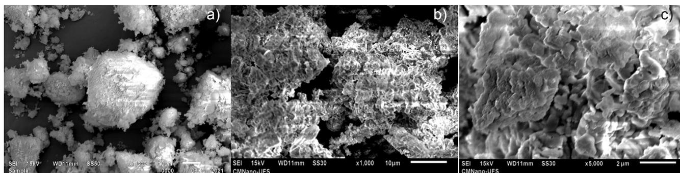
Figure 4: SEM micrographs of the soil (a) and wood ash particles (b,c).
