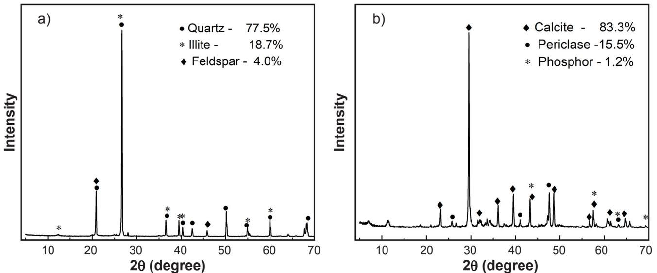
Figure 3: X-ray diffraction patterns of the soil (a) and wood ash (b).
