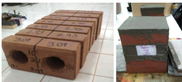
Figure 1: Preparation of the bricks for the compressive strength test.
