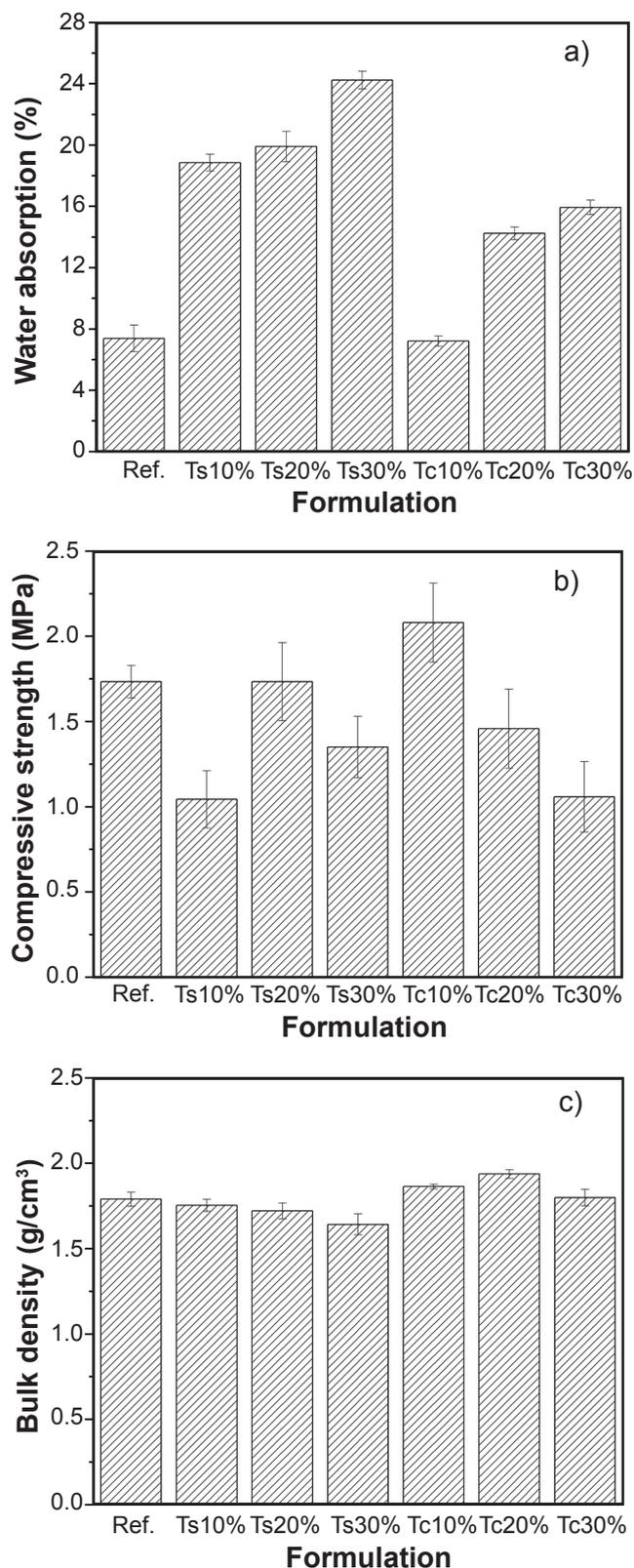
Figure 5: Results of water absorption (a), compressive strength (b), and bulk density (c) of the bricks.
