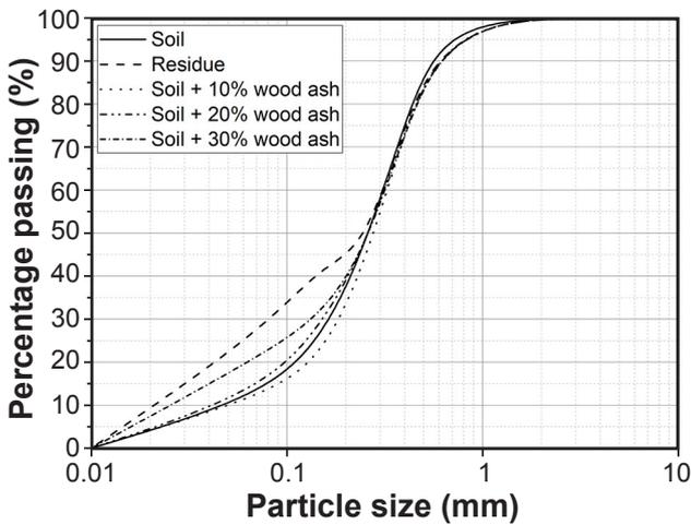
Figure 2: Granulometric curves of the soil, wood ash, and mixtures.
