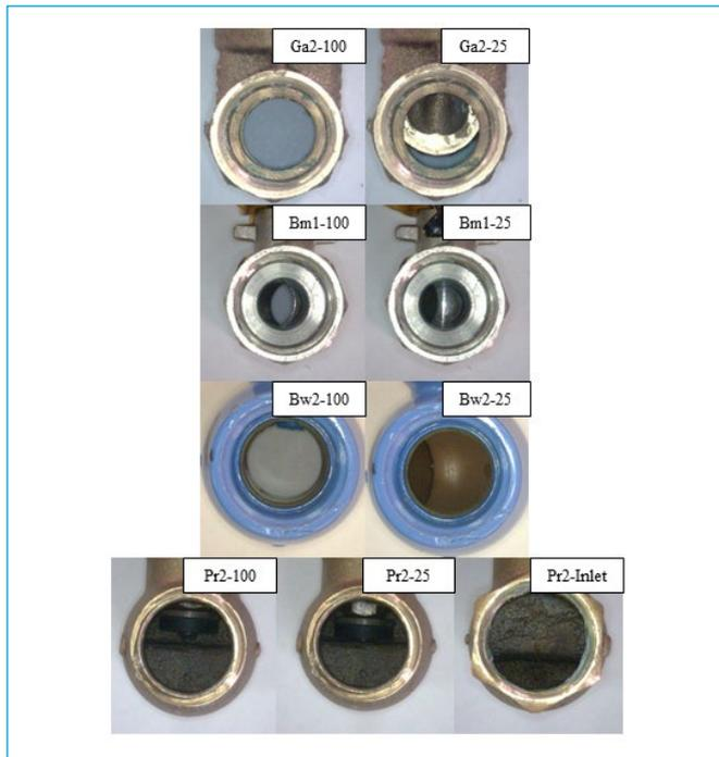
Figure 2 - Constructive and flow section specificities for some of the evaluated valves with 100 and 25% openings, and inlet detail of pressure valves.
