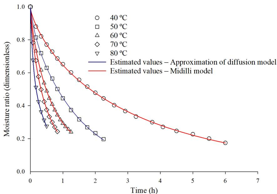
**Figure 2:** Moisture ratios estimated using Midilli and the Approximation of diffusion models for the drying of buckwheat (*Fagopyrum esculentum* Moench) grains at different drying air temperatures.
