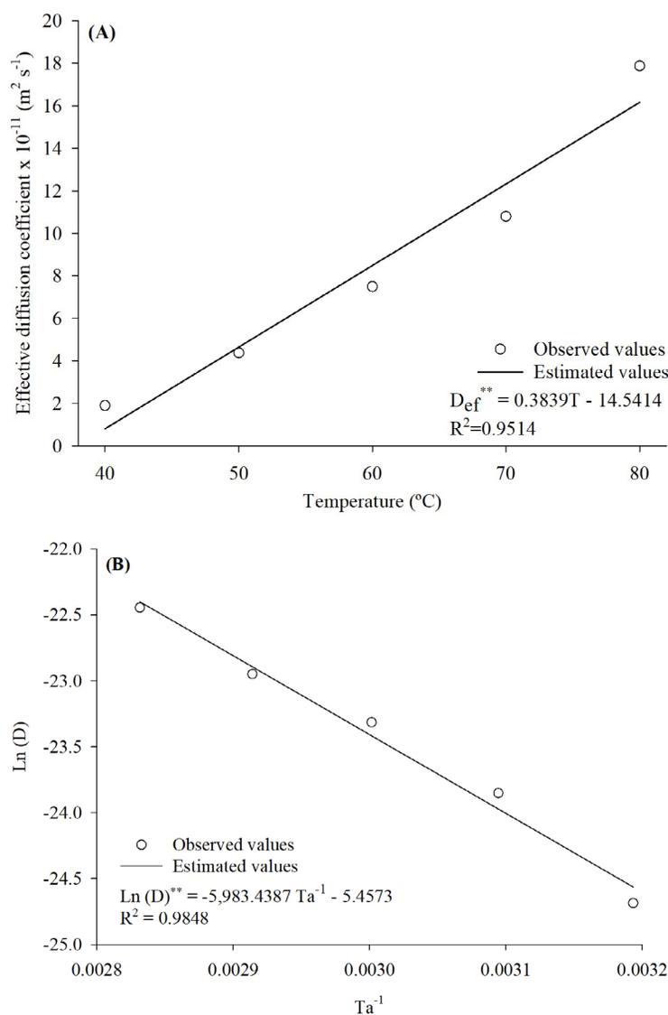
**Figure 3:** Average values of the effective diffusion coefficient (A) and the Arrhenius representation of the effective diffusion coefficient (B) at different drying air temperatures for buckwheat (*Fagopyrum esculentum* Moench) grains (\*\*significant at 1%, using the t-test).
