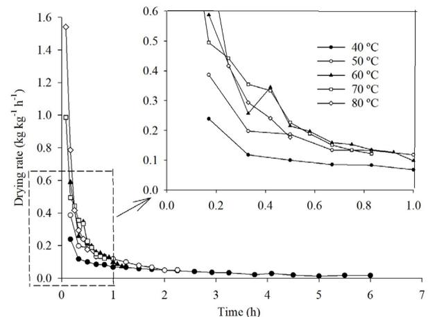
**Figure 1:** Moisture reduction rates for buckwheat grains at different drying air temperatures.
