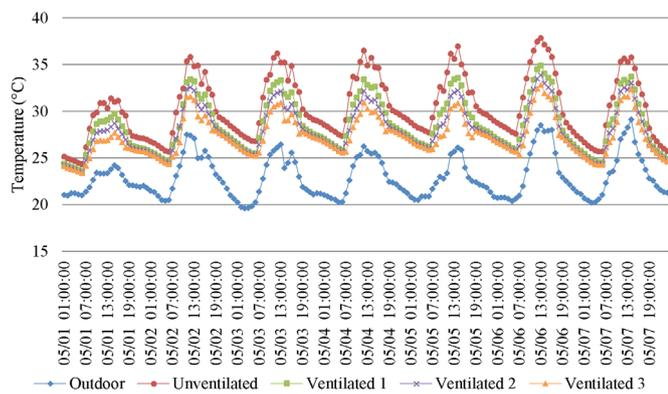
Figure 5. Thermal behavior - solar dryer of coffee - second floor - first week
