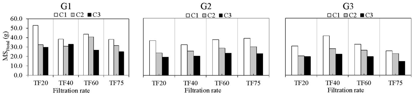
Figure 3. Behavior of total mass of solids present in the filter bed after filtration (before backwashing) ( $MS_{Ftotal}$ ), for different combinations of sand granulometry (G1, G2 and G3), filtration rates (TF20, TF40, TF60 and TF75) and filtration cycles (C1, C2 and C3)
