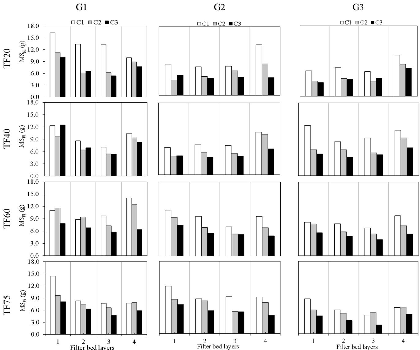
Figure 2. Behavior of mass of solids present in the filter bed after filtration (before backwashing) in different filter bed layers ( $MS_{Fi}$ ) for different combinations of sand granulometry (G1, G2 and G3), filtration rates (TF20, TF40, TF60 and TF75) and filtration cycles (C1, C2 and C3)
