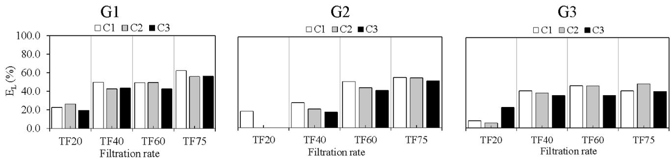
Figure 5. Behavior of cleaning efficiency considering the entire filter bed ( $E_L$ ), as a function of different filtration cycles (C1, C2 and C3), sand granulometries (G1, G2 and G3) and filtration rates (TF20, TF40, TF60 and TF75)
