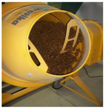
Figure 1. Mixture homogenized in concrete mixer
