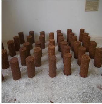
Figure 2. Specimens healing in open air
