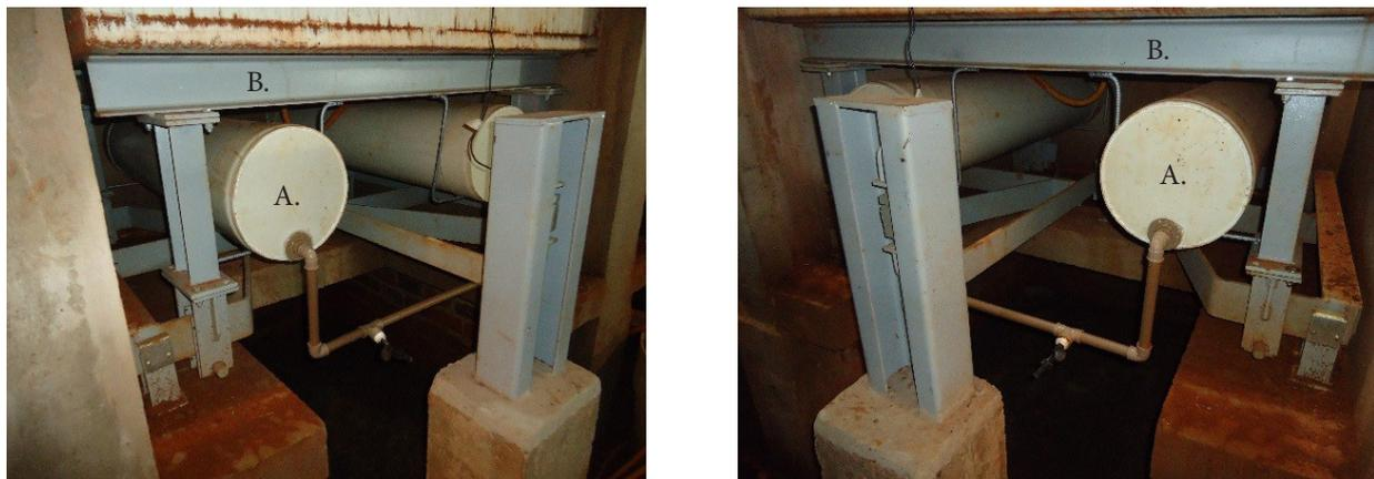
**Figure 3.** Drainage system (A) of weighing lysimeters fixed on the upper frame (B) of the set of levers
