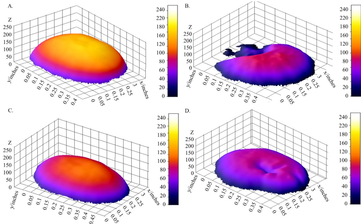
**Figure 2.** The three-dimensional pixel density graphs plot for the seeds that were obtained from manual processing (full and well-formed seeds – A; and with endosperm and cotyledons damage - B); together with the mechanically processed seeds (filled and well-formed seeds– C; with damage to the seed hilum and the embryo - D)
