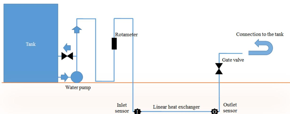
**Figure 2.** Schematic model for the passage of water through the linear heat exchanger
