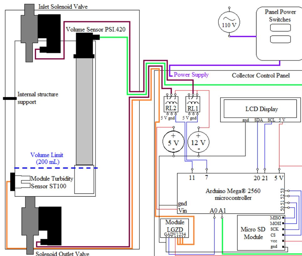
**Figure 1.** Internal schematic of the prototype showing the position of the sensors, structural schematic of the collector, and electrical configuration of the control panel
