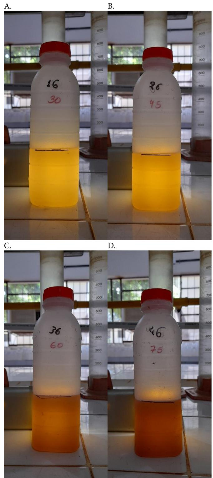
**Figure 2.** Runoff samples representing the rainfall intensities of 30 (A), 45 (B), 60 (C) and 75 mm h<sup>-1</sup> (D) applied by the rainfall simulator in the field
