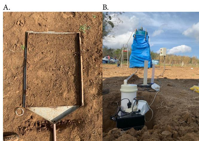
**Figure 4.** Structure of the collector plot (0.70 m<sup>2</sup>) (A) and collector installed in the field next to the InfiAsper simulator (B)
