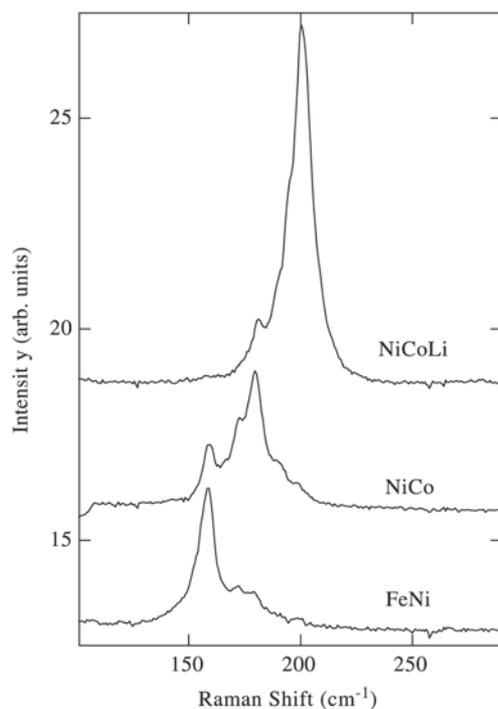
**Figure 3.** Raman spectra from three different SWCNTs samples in the radial breathing mode frequency range.
