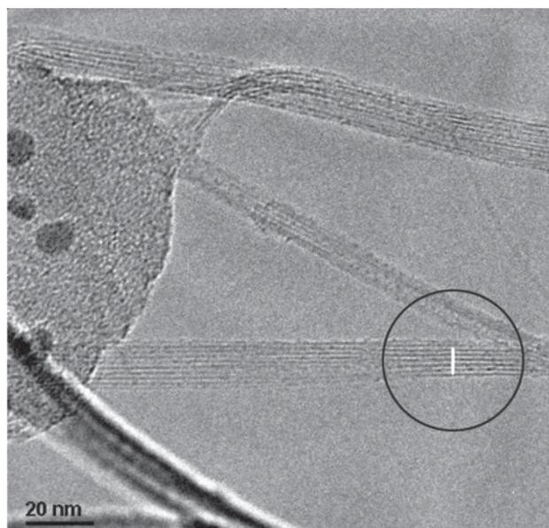
**Figure 2.** High magnification HRTEM image of SWCNTs produced using the catalyst mixture:  $\text{LiNi}_{0.5}\text{Co}_{0.5}\text{O}_2$  and the arc-discharge method.
