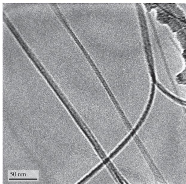
**Figure 1.** High Resolution Transmission Electron Microscopy of SWCNTs produced using the catalyst mixture:  $\text{LiNi}_{0.5}\text{Co}_{0.5}\text{O}_2$  and the arc-discharge method.
