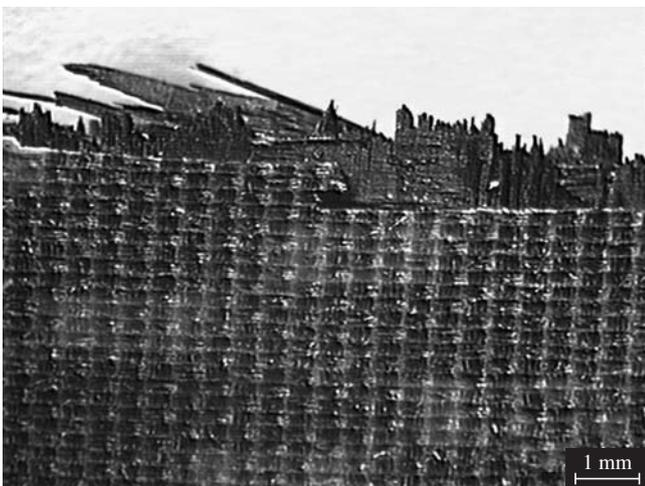
Figure 10. F155/8HS specimen after tensile test, (10x).
