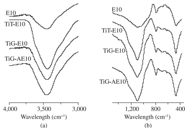
**Figure 6.** IR spectra of the montmorillonite clay E with and without OH-Ti treatments after thermal treatment at 1,000 °C.
