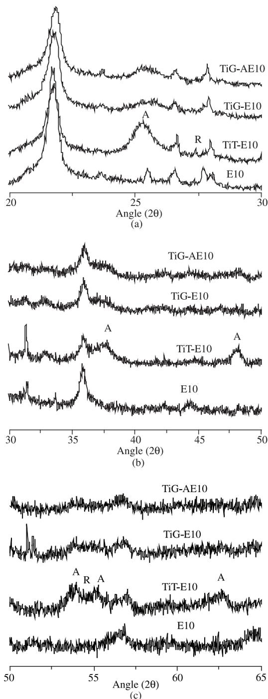
**Figure 5.** XRD diagrams of the montmorillonite clay E with and without OH-Ti treatments after thermal treatment at 1,000 °C.
