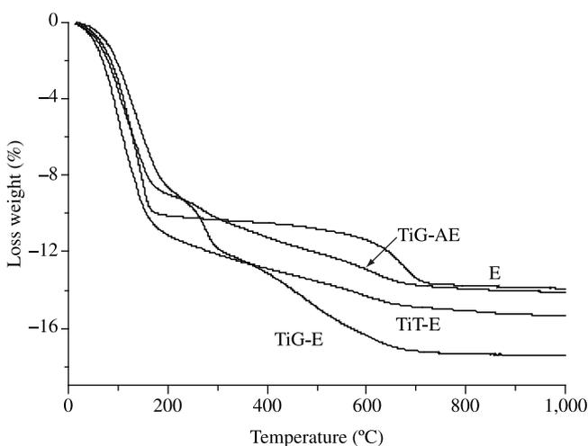
**Figure 2.** TG diagrams of the montmorillonite clay E with and without OH-Ti treatments.
