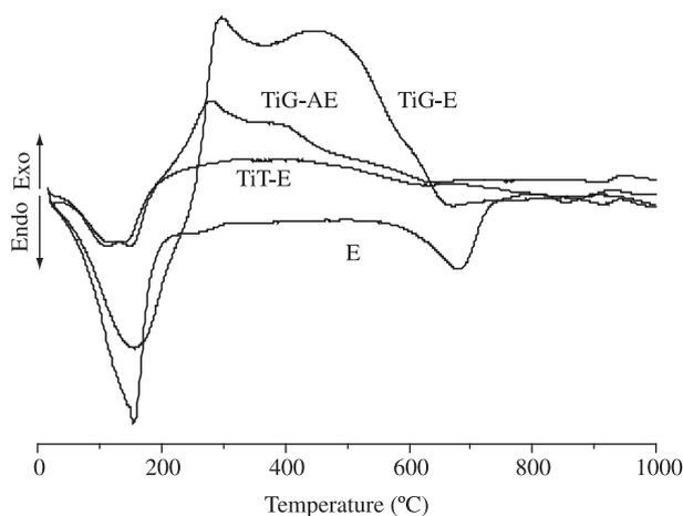
**Figure 1.** DTA diagrams of the montmorillonite clay E with and without OH-Ti treatments.
