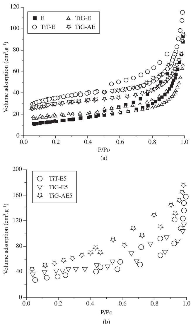
**Figure 3.** N<sub>2</sub> adsorption-desorption isotherms of the montmorillonite clay E with and without OH-Ti treatments. a) in natural conditions; and b) after thermal treatment at 500 °C.
