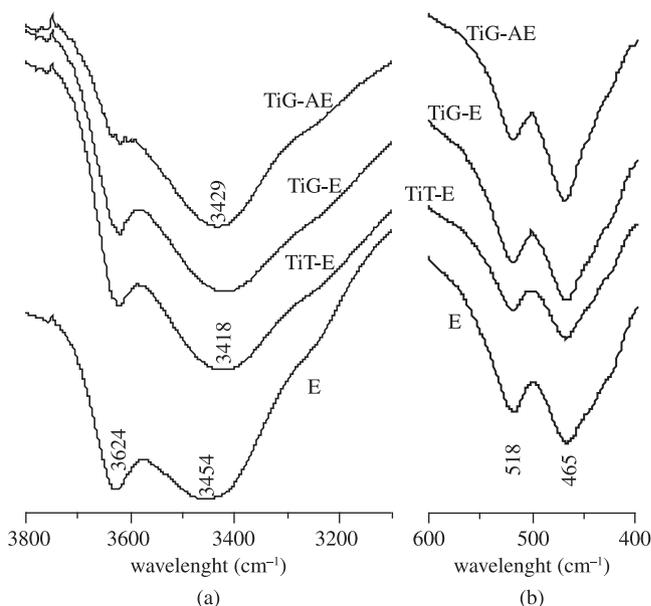
**Figure 4.** IR spectra of the montmorillonite clay E with and without OH-Ti treatments.
