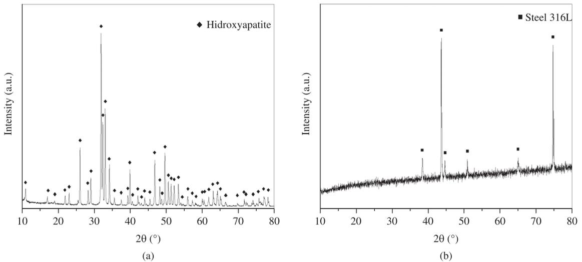
**Figure 2.** X-ray diffraction patterns of raw materials used in preparation of biocomposite 316L/HA: a) hydroxyapatite powder b) powder of stainless steel 316L.
