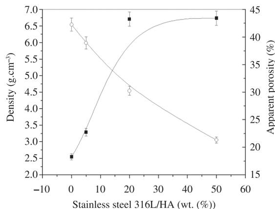
**Figure 6.** Density and apparent porosity of different compositions of the biocomposite stainless steel 316L/HA (5, 20 and 50 wt. (%) HA).
