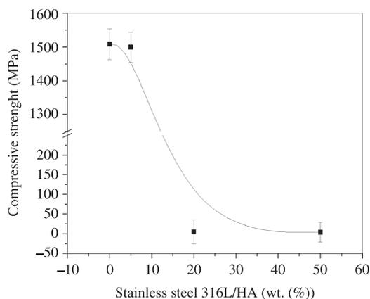
**Figure 7.** Mechanical properties (compressive strength) of different compositions of the biocomposite stainless steel 316L/HA (5, 20 and 50 wt. (%) HA).
