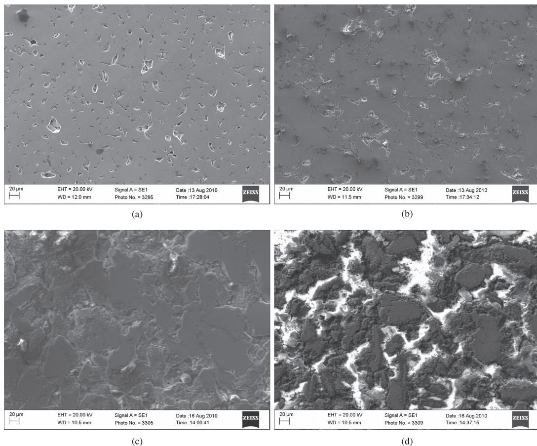
**Figure 4.** SEM micrographs of different compositions of the biocomposite steel 316L/HA: a) pure stainless steel b) 5 wt. (%) HA, c) 20 wt. (%) HA and d) 50 wt. (%) HA.
