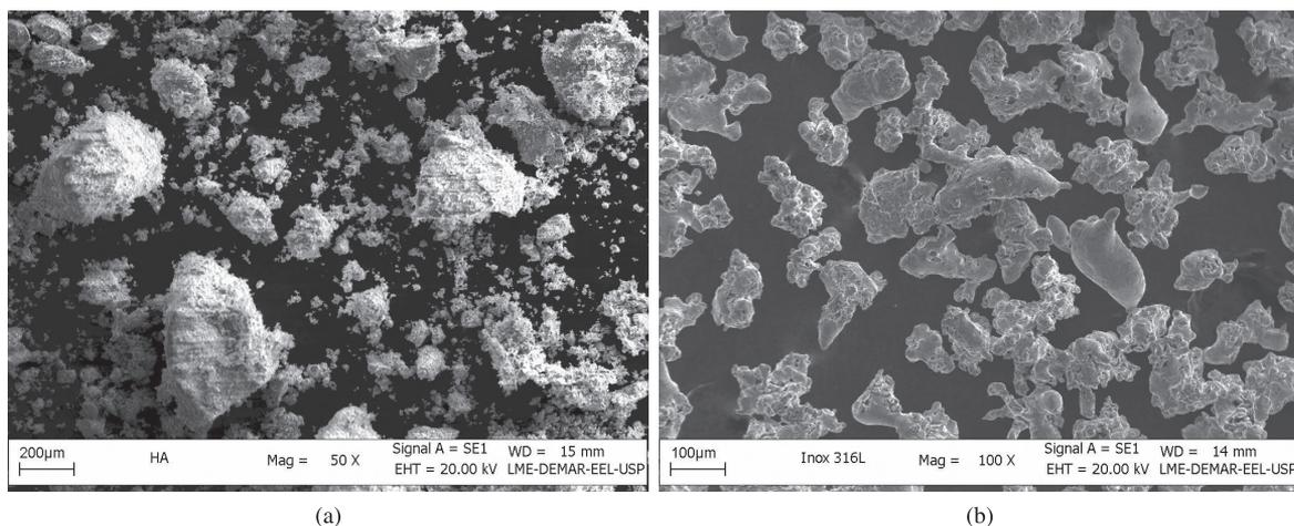
Figure 1. SEM micrographs shown the morphology of the powder particles of: a) HA and b) 316L stainless steel.
