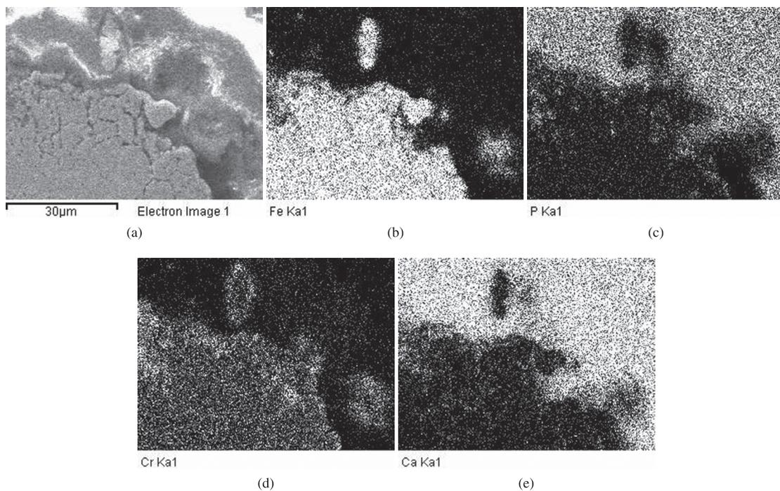
**Figure 5.** Mapping carried at the interface of the sample with 50 wt. (%) HA after sintering a) analyzed region, b) distribution of Fe, c) distribution of P d) distribution of Cr and e) distribution of Ca.
