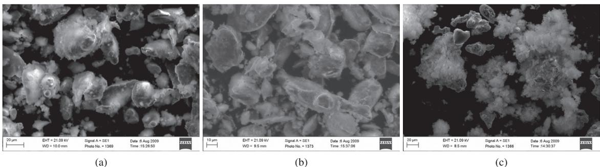
**Figure 3.** SEM micrographs of the different powder mixtures milled for 10 hours: a) 5 wt. (%) HA, b) 20 wt. (%) HA and c) 50 wt. (%) HA.
