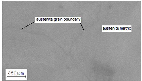
Figure 7. Optical micrograph of sample of sound crusher jaw(s) showing austenite grain boundaries in austenite matrix.
