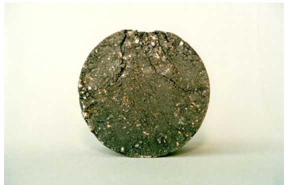
Figure 3. The general view of the Soma fly ash (F type) modified specimen after failure at the end of the carried out repeated load indirect tensile test.
