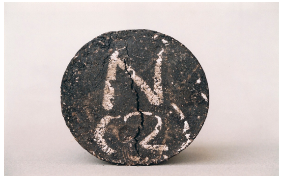
Figure 2. The general view of the control specimen after failure at the end of the carried out repeated load indirect tensile test.
