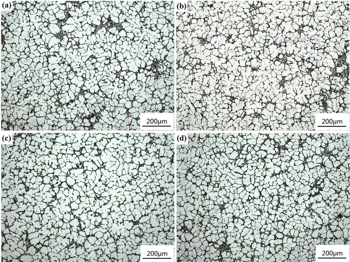
**Fig. 4** Microstructures of semi-solid ZL101 aluminum alloy slurry prepared by serpentine channel with 4 curves at different temperatures (a) 690°C; (b) 670°C; (c) 650°C; (d) 630°C
