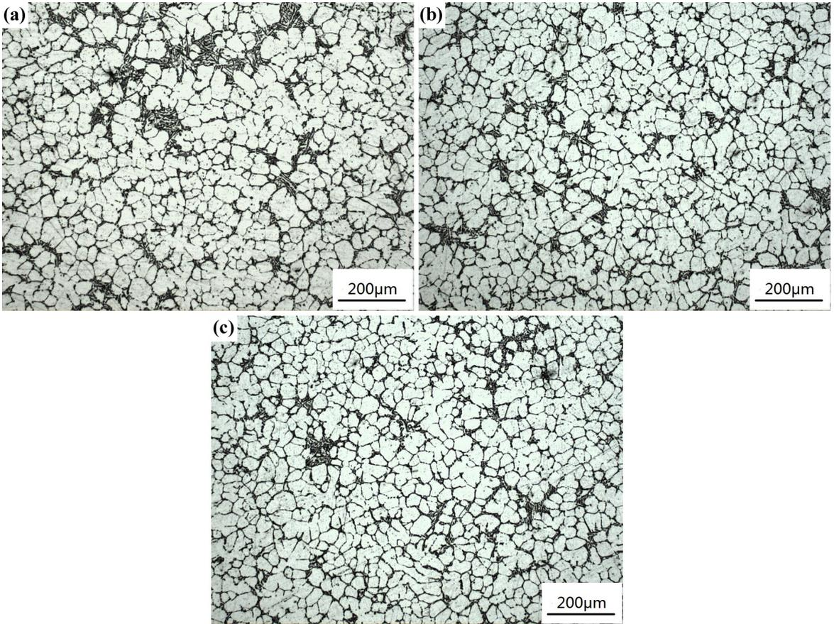
**Fig. 6** Microstructures of semi-solid ZL101 aluminum alloy slurry prepared by serpentine channel with different curve numbers at 630°C (a) 3 curves; (b) 4 curves; (c) 5 curves
