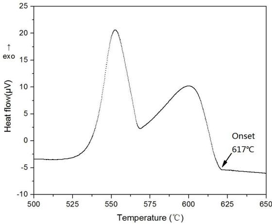
Fig. 1 DSC cooling curves of ZL101 aluminum alloy
