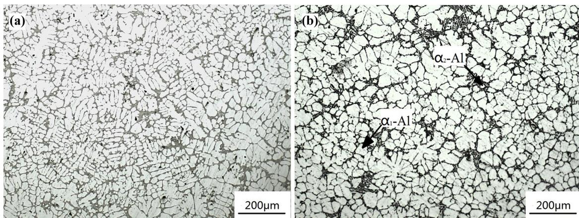
Fig. 3 Microstructures of ZL101 aluminum alloy slurry prepared by two methods (a) conventional casting; (b) serpentine channel
