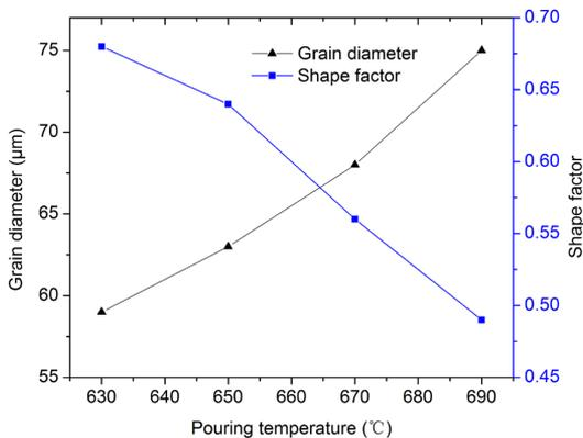
**Fig. 5** Effects of pouring temperature on  $D$  and  $S_f$
