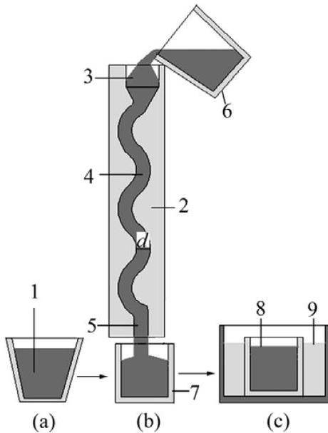
Fig. 2 Schematic diagram of preparing semi-solid ZL101 aluminum alloy slurry by serpentine channel: (a) Melt; (b) Preparation of semi-solid slurry; (c) Cooling. 1—K-type thermocouple; 2—Serpentine channel; 3—Pouring cup; 4—Serpentine bend; 5—Diversion pipe; 6—Melting crucible; 7—Collective crucible; 8—Slurry; 9—Cold water
