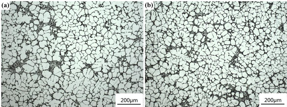
**Fig. 8** Microstructures of semi-solid ZL101 aluminum alloy slurry prepared by serpentine channel with different temperature: (a) 100°C; (b) 25°C
