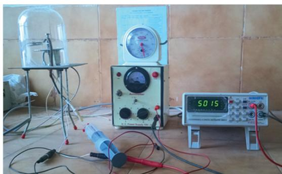
Figure 1. Photographic view of gas sensing setup.
