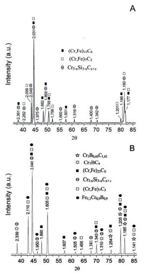
**Figure 4:** XRD diffraction patterns of the coatings. A) - Chromizing and B) - Chrome–boronizing–siliconizing (obtained using the mixture 2).
