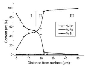
Figure 3: Concentration profiles of chromium, iron and silicon (by EDS) in the cross section of a sample chrome–boronizing–siliconizing (obtained using the mixture 3).
