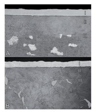
**Figure 5:** Cross-sectional morphology of the coatings (Optical Microscopy), 500 X. A - Chromizing, B - Chrome–boronizing–siliconizing (obtained using the mixture 3).
