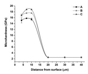
Figure 6: Cross-sectional microhardness profiles. A - Chromizing, B - Chrome–boronizing–siliconizing (obtained using the mixture 2) and C - Chrome–boronizing–siliconizing (obtained using the mixture 3).
