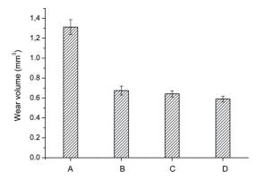
**Figure 8:** Wear volume. A - Heat treatment, B – Chromizing, C – Chrome-boronizing-siliconizing (obtained using mixture 2) and D - Chrome-boronizing-siliconizing (obtained using mixture 3).
