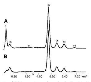
Figure 2: EDS spectra of the coatings surface. A - Chromizing, B - Chrome–boronizing–siliconizing (obtained using the mixture 3).
