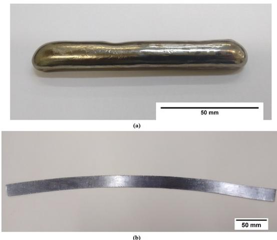
**Figure 1.** (a) Ingot and (b) plate obtained after rolling
