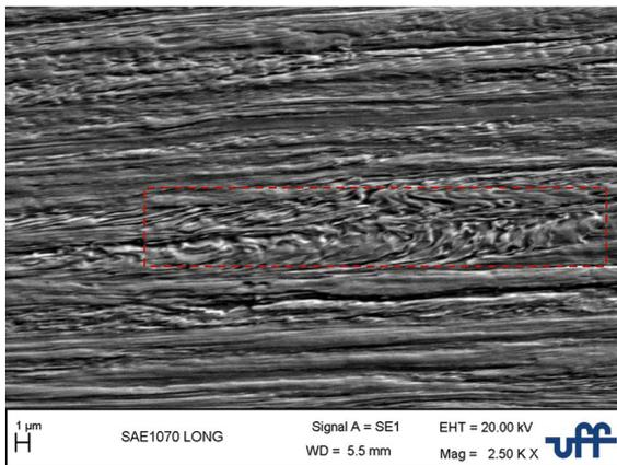
**Figure 4.** SEM. Longitudinal section of SAE 1070 steel cold-deformed with accumulated strain of 2.52.
