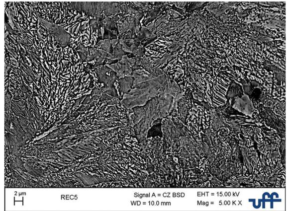
**Figure 5.** SEM. Cross section of SAE 1070 steel annealed at 1000°C for 5 min.
