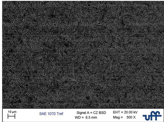
**Figure 2.** SEM. Cross section of SAE 1070 steel cold-deformed with accumulates strain of 2.52.
