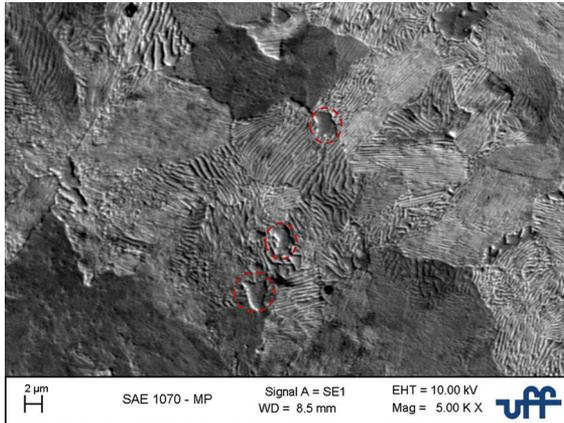
**Figure 1.** SEM. Cross section of SAE 1070 steel in the initial condition.
