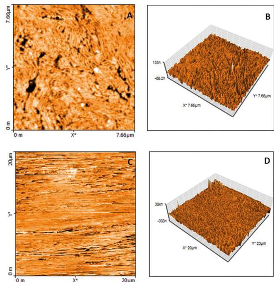
**Figure 3.** AFM. Micrograph of SAE 1070 steel, cold-deformed with accumulated strain of 2.52 (A) cross section and (C) longitudinal section. Topography of SAE 1070 steel, cold-deformed with accumulated strain of 2.52 (B) cross section, with the analyzed area of 58.6756  $\mu\text{m}^2$  and (D) longitudinal section, with the analyzed area of 400  $\mu\text{m}^2$ .
