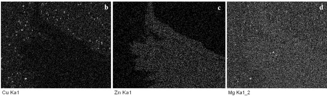
**Figure 6.** Spectrum of alloy elements distribution and mixture zone appearance obtained by SEM.
