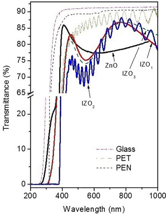
**Figure 3.** The optical transmittance of the ZnO, IZO films and the PEN, PET and glass substrates.
