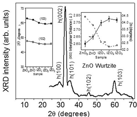
**Figure 1.** XRD diffractogram of an IZO representative film. The film crystallized in the hexagonal wurtzite phase with preferential orientation in the (002) direction. The insets show shifts in the interplanar distance and diffraction peak position as a function of the IZO films.
