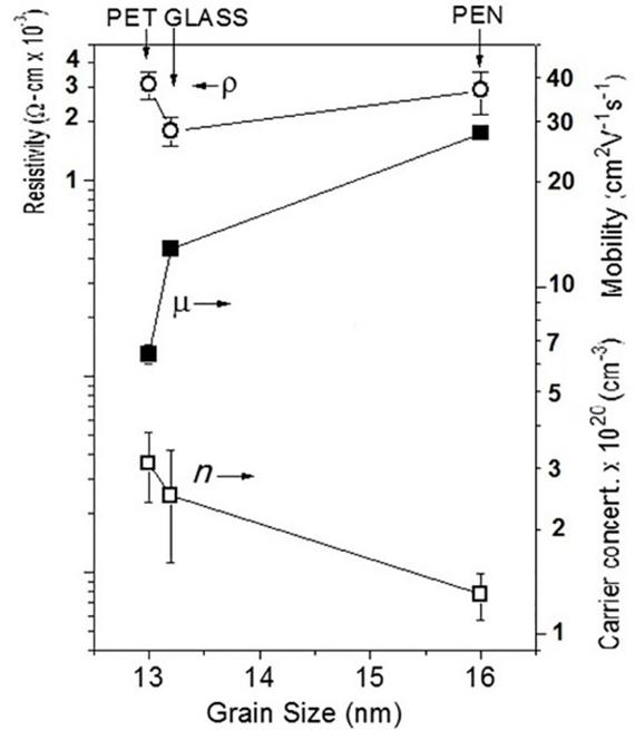
**Figure 4.** Resistivity ( $\rho$ ), Mobility ( $\mu$ ) and Carrier concentration ( $n$ ) behavior as a function of the grain size ( $GS$ ) for the IZO samples. From the graph and results in Table 2 note electrical parameters change considerably compared with those measured in the reference ZnO sample. The inset shows the ZnO unit cell.
