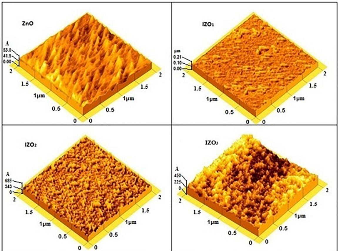
Figure 2. AFM images of ZnO and IZO films deposited on different substrates at RT by rf magnetron sputtering.
