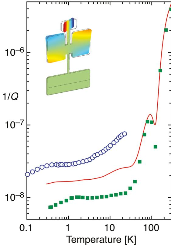
**Figure 1.** Inverse Quality Factor ( $Q^{-1}$ ) versus Temperature for original DPO (blue open circles), our standard DPO (red solid curve), and a recent DPO (green solid squares). Inset: illustration of DPO resonator. Color scale indicates out-of-plane displacement at AS2 oscillation maximum; wireframe shows equilibrium position.
