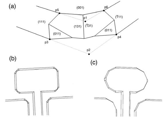
**Figure 3.** (a) Illustration of exterior corner of a DPO, with crystallographic faces and some of the points used in the construction labeled. (b) Close-up of head of a DPO with corners etched to Etch Parameter 1.5. (c) Close-up of head of DPO with corners etched to Etch Parameter 4.5.
