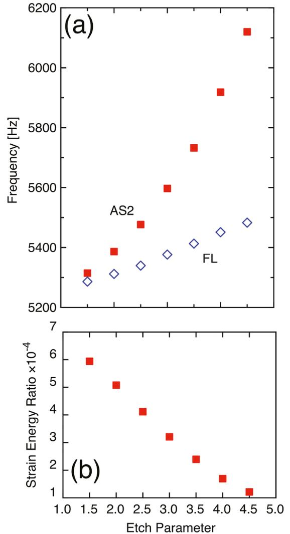
**Figure 5.** (a) Frequency of AS2 (red solid squares) and FL (blue open diamonds) modes as a function of Etch Parameter, for FEM modeled DPOs. (b) Ratio of strain energy in foot to total strain energy in DPO, as a function of Etch Parameter. Note  $10^{-4}$  scaling of ratio.
