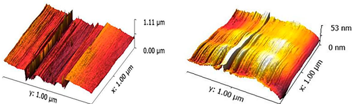
**Figure 5.** Atomic force microscopy of the PEEK porous (a) and smooth (b) surface, respectively.
