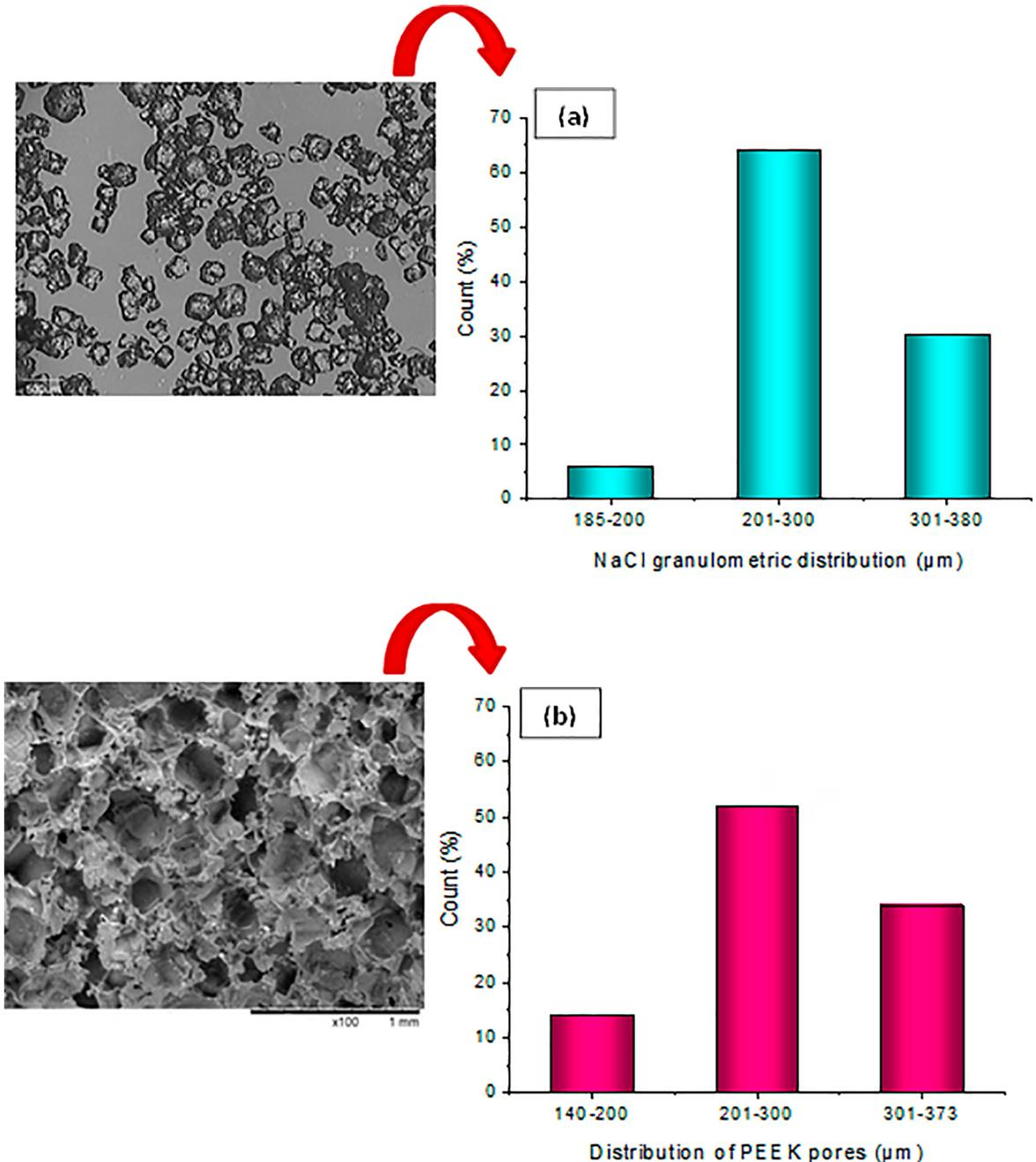
**Figure 3.** Histograms of NaCl granulometric distribution (a) and distribution of PEEK porous (b) measured with ImageJ software.
