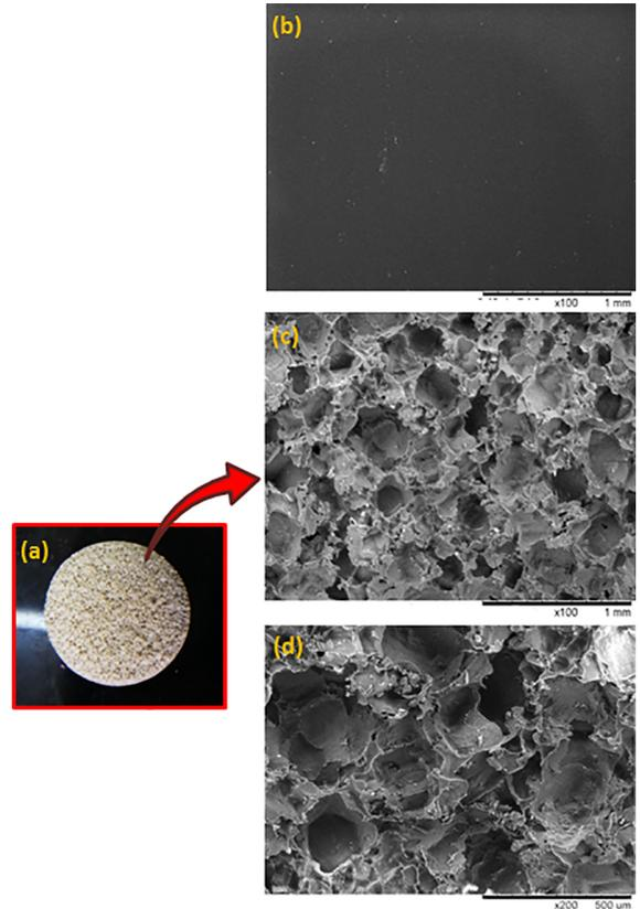
**Figure 1.** Micrographs of the porous surface of the sample without magnification (a), surface without pores with magnification of 100x (b), surface porous with magnification of 100x (c) and with magnification 200x (d).
