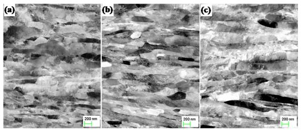
Figure 1. AsB maps of a 0.17C-6.6Mn-1.1Al-0.05Nb-0.22Mo steel processed by warm rolling at various temperatures: (a) 630 °C, (b) 660 °C and (c) 690 °C.
