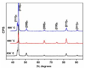
**Figure 4.** X-ray diffraction patterns of a 0.17C-6.6Mn-1.1Al-0.05Nb-0.22Mo steel processed by warm rolling at temperatures ranging from 630 to 690 °C.
