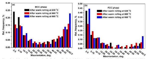
Figure 3. Grain boundaries misorientation distribution profiles for both BCC(a) and FCC(b) phases in a 0.17C-6.6Mn-1.1Al- 0.05Nb-0.22Mo steel processed by warm rolling at 630, 660 and 690 °C.
