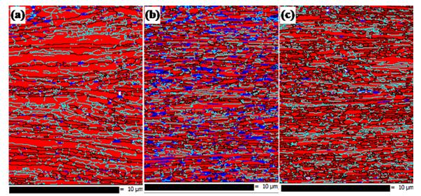
Figure 2. Phase distribution and grain boundaries of a 0.17C-6.6Mn-1.1Al-0.05Nb-0.22Mo steel processed by warm rolling at various temperatures: (a) 630 °C; (b) 660 °C and (c) 690 °C. BCC-red; FCC-blue; HAGBs (>15°)-solid black line; LAGBs (2~15°)-solid green line.
