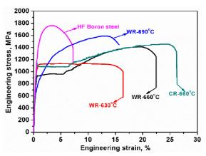
Figure 5. Engineering stress-strain curves of a 0.17C-6.6Mn-1.1Al-0.05Nb-0.22Mo steel processed by warm rolling at temperatures ranging from 630 to 690 °C, together with those of HFed 22MnB5 steel [4] and the CRed specimen after annealing at 660 °C for 30 min [7].
