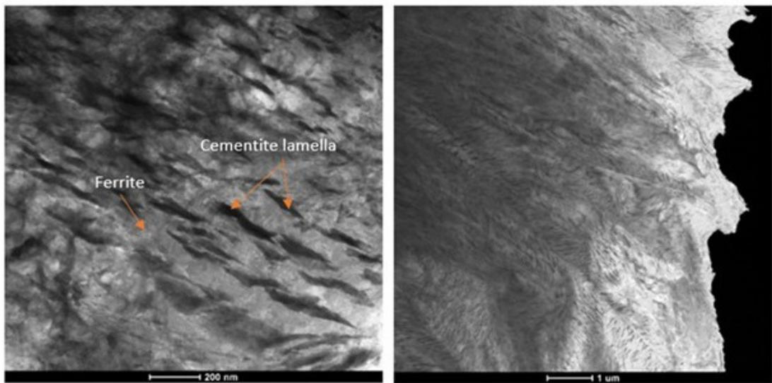
**Figure 22.** *Nb2 steel*: TEM images of Charpy specimens in section B and position 4 (wheel flange area), tempered at 300 °C (7J). Minimum Charpy result inside the embrittlement area. Microstructure is fully bainite (B).
