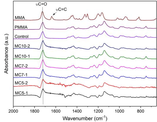
Figure 1. FTIR spectra of MMA, PMMA, Control, MC5, MC7 and MC10.
