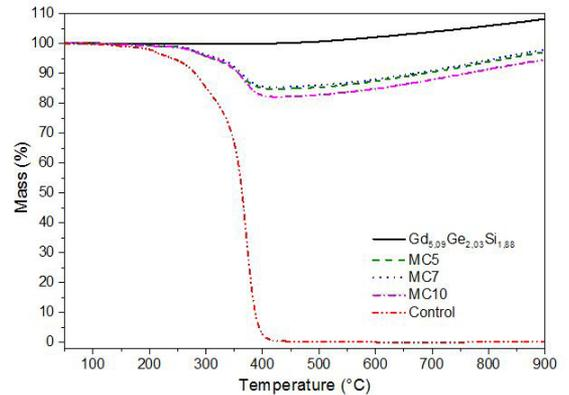
Figure 2. Thermogravimetric curve of  $Gd_{5.09}Ge_{2.03}Si_{1.88}$  powder, MC5, MC7, MC10 and Control.
