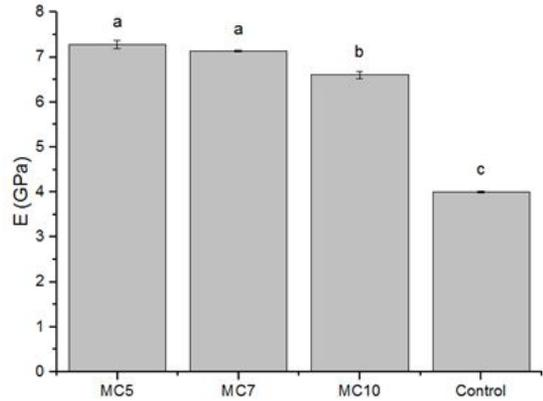
**Figure 5.** The elastic modulus of the magnetocaloric composites and control sample. Different letters indicate statistical differences between the samples.
