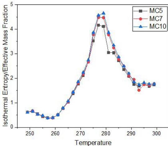
**Figure 8.** Effective PMMA mass fraction influence on the isothermal variation entropy [ $\Delta S_T/PMMA(g)$ ] for various compositions.
