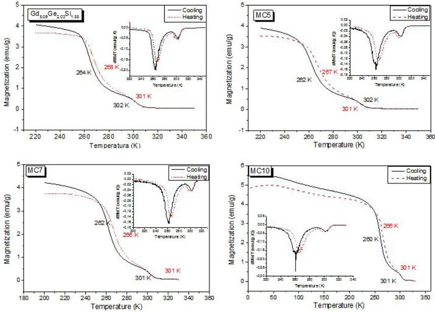
**Figure 6.**  $M$  vs.  $T$  measurements of  $Gd_{5.09}Ge_{2.03}Si_{1.88}$  powder, MC5, MC7 and MC10. The insets on the graphs are the derivatives of the curves.
