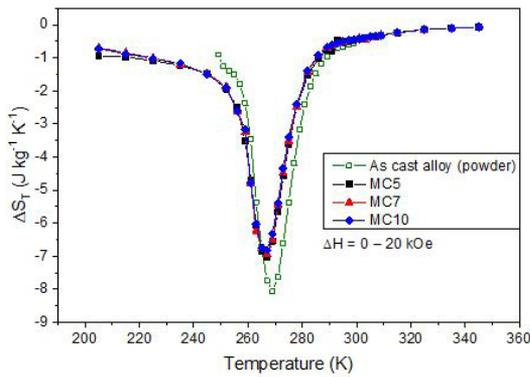
**Figure 7.** Isothermal variation of entropy ( $\Delta S_T$ ) at a magnetic field variation from 0 to 20 kOe for  $Gd_{5.09}Ge_{2.03}Si_{1.88}$  powder, MC5, MC7 and MC10.
