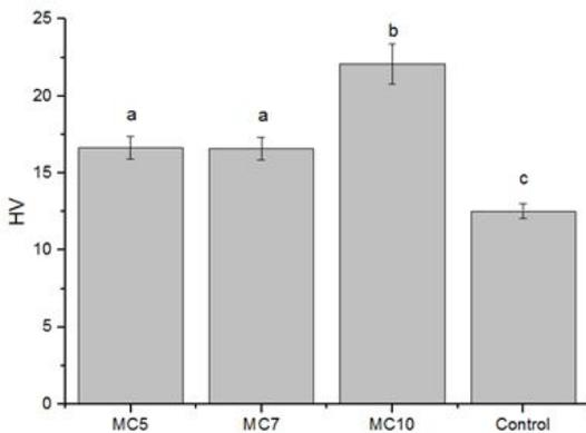
**Figure 4.** Vickers hardness of the magnetocaloric composites and control sample. Different letters indicate statistical differences between the samples.
