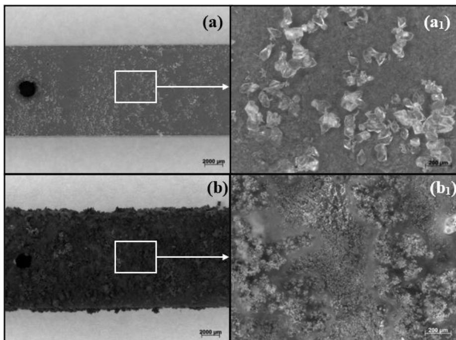
**Figure 4.** Macrographs of the film and biofilm formed on the coupon surface after 15 days of exposure to abiotic (a and a<sub>1</sub>) and biotic (b and b<sub>1</sub>) systems, respectively. Magnification of 7x (a and b) and 100x (a<sub>1</sub> and b<sub>1</sub>).
