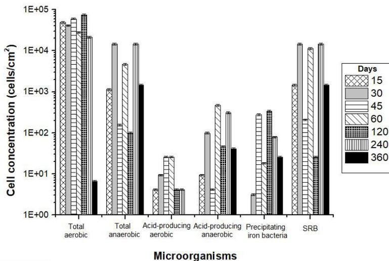
**Figure 3.** Cellular concentration of sessile microorganisms quantified by the Colony Forming Unit (CFU) and Most Probable Number (MPN) techniques.
