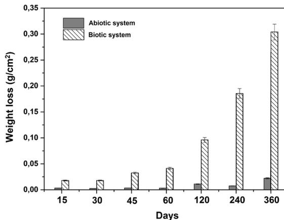
Figure 6. Weight loss of coupons X80 in produced water.
