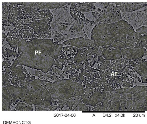
**Figure 1.** Microstructure showing acicular ferrite (AF) and polygonal ferrite (FP) of X80 steel (magnification 4000x).
