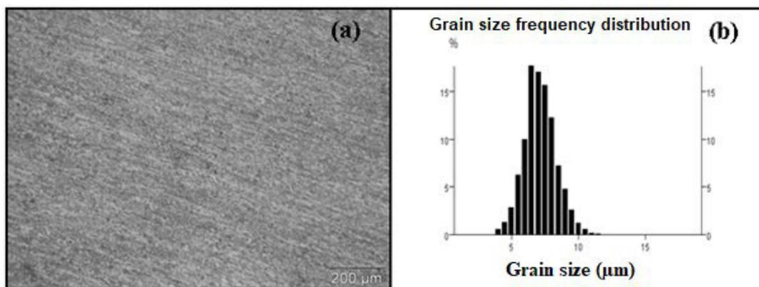
**Figure 2.** Grain size distribution of X80 steel. In (a) micrograph of the coupon with 100x magnification and (b) grain size graph versus percentage referring to the grain size.
