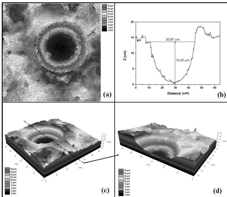
**Figure 7.** Pit formed on the surface of the X80 steel coupon after 45 days of exposure to the biotic system. In (a) 2D analysis, (b) profile of the pit, (c) 3D topography and (d) cross section of the pit in 3D
