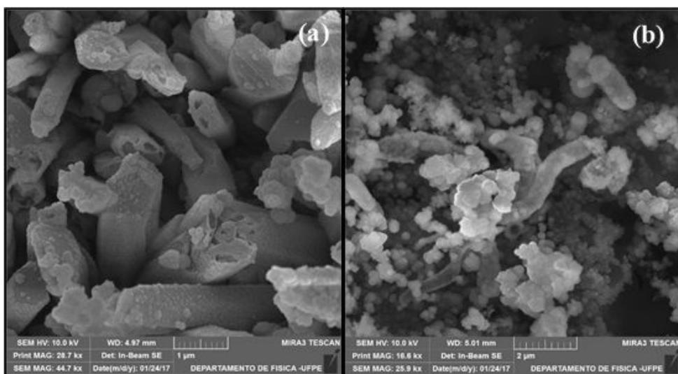
**Figure 5.** Micrographs of the film and biofilm formed on the coupon surface after 15 days of exposure to (a) abiotic and (b) biotic systems. Magnification of 44.700x (a) and 25.900x (b).
