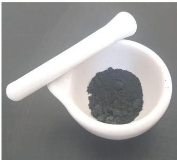
Figure 1. CRFO after calcination.
