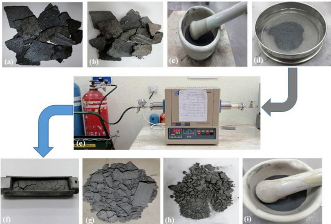
**Figure 2.** Schematic representation of the reduction procedure with used tools and equipment's; (a) Mill scale, (b) Mill scale after drying at 250°C, (c) Hand mill, (d) Sieving process, (e) Tube furnace with H<sub>2</sub> gas system, (f) Produced iron powder, (g), (h), (i) preparation of produced iron powder.
