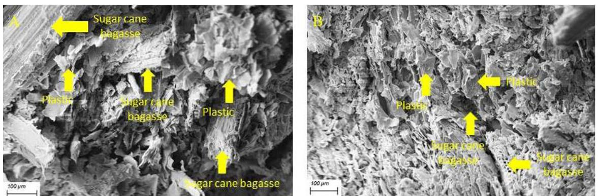
**Figure 4.** Images obtained by scanning electron microscopy for panels produced at 160°C (A) and 220°C (B).
